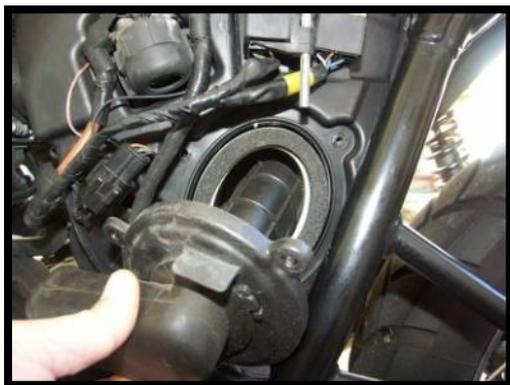
4) Replace the OEM cover/snorkel with the Breathe cover and don't forget to swap the large sealing O ring from the OEM cover to the Breathe.
