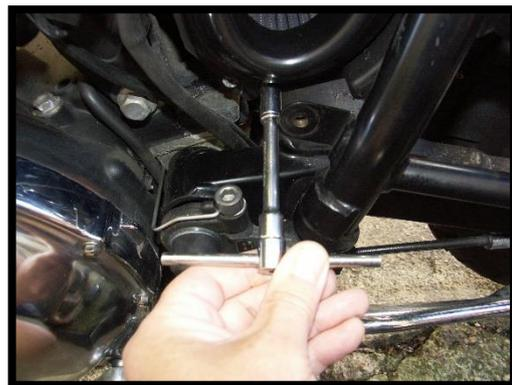
5) Replace the three OEM 8mm bolts in the Breathe cover and tighten to 3 Nm.
