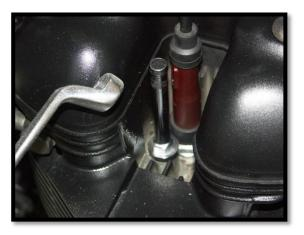
8) Use a 13mm ring spanner remove both the chrome tubes, apply some copper grease to the threads of the alloy bung, place a copper washer on the bung and with a 6mm hex key/socket torque to Triumph specs. Repeat for the other side.
