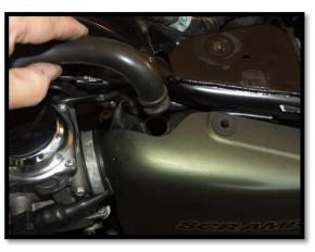
4) Pull away the large rubber hose that sucks air from the air box and seal the hole with the supplied plastic bung.
