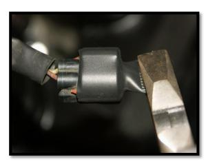
5) **EFI MODELS**: Unplug the electrical connector from the SAI unit and place the supplied heat shrink over the remaining loom electrical connector and use a heat gun to shrink to size. With the heat shrink still hot, clamp the open end with a pair of pliers to seal from the elements. **Do not** use your fingers, the heat shrink is far too hot.
